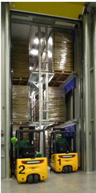
Three-storey ripening chamber
