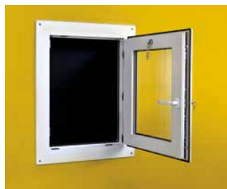
Integrated gastight ULO window. Custom built with key lock and 1-handle system for emergency escape. Pivot fitting with 10-point locking mechanism.
